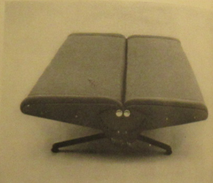
"The chair of the Tenth Triennale"—architect Carlo de Carli's featherweight chair is connected by exposed brass screws. Under the shell-thin, molded plywood seat a pair of metal reinforcing rods criss-cross. They too are held by the seat screws, come flat when the chair is demounted.
