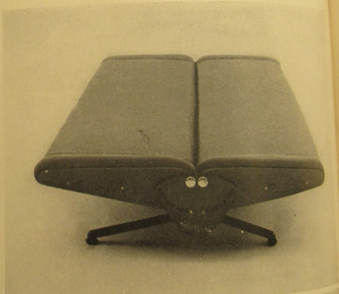
"The chair of the Tenth Triennale"—architect Carlo de Carli's featherweight chair is connected by exposed brass screws. Under the shell-thin, modular plywood seat a pair of metal reinforcing rods criss-cross. They too are held by the seat screws, come flat when the chair is demounted.
