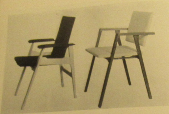
"The chair of the Tenth Triennale"—architect Carlo de Carli's featherweight chair is connected by exposed brass screws. Under the shell-thin, molded plywood seat a pair of metal reinforcing rods criss-cross. They too are held by the seat screws, come flat when the chair is demounted.
