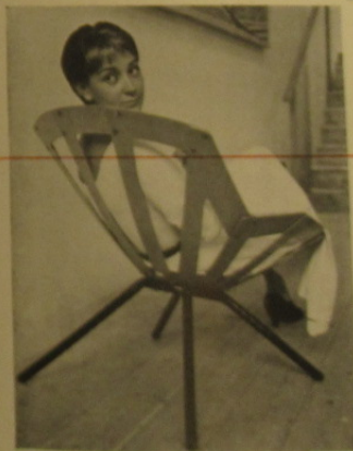
Two chairs by architects Gregotti, Meneghetti and Stoppino (Nocera factory) exploit flexibility of plywood without expensive molding. Above: Scoop made of 12 L-shaped pieces of plywood, flexing under sitter's weight and spreading the load, so extremely thin plywood is sufficient. Comes also with separate, well-filled foam cushions. Right: This plywood sheets, with strategic incisions, flex at back and seat.
